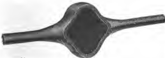
Fig. 4.—One-piece pressed steel rear axle housing.
